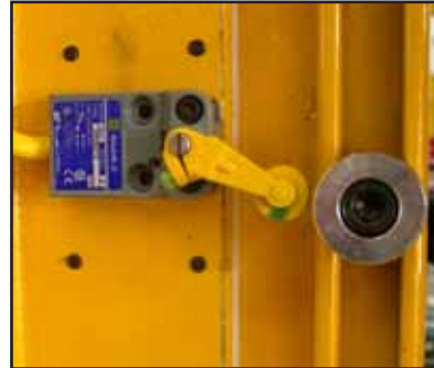
Figure 7-2: Limit Switch and Puck
